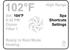
**Rest Mode** will only allow heating during programmed filter cycles. Since polling does not occur, the temperature display may not show a current temperature until the filtration pump has been running for a minute or two. **Ready in Rest Mode** may appear when Jets 1 is activated.
